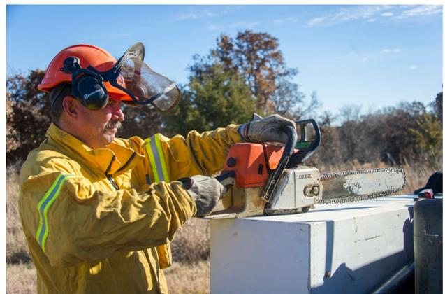
When using a chainsaw, safety should be your top priority. Chainsaw operators should wear full protective gear. Care should be taken when operating the chainsaw near hot spots on the tree due to the air movement created by the saw, which can cause flames to flare-up injuring the operator or damaging the saw. (Photo courtesy T. Johnson)
