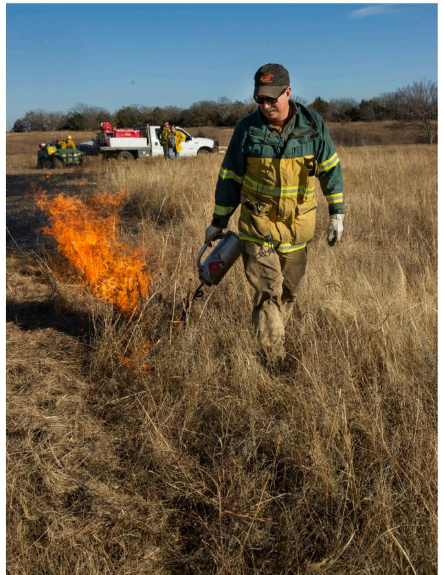
**The most widely used ignition device is a drip torch. Drip torches use a mixture of diesel and gasoline. A mixture of 50:50 diesel to gasoline works very well for temperatures ranging from 35 F to 75 F. When temperatures are higher than this, a mixture of 60:40 or 70:30 diesel to gasoline is recommended to reduce the volatility of the gasoline and to help the torch operate properly.** (Photos courtesy: J. Weir top and bottom left, J. Bradley top right, T. Johnson bottom right)
